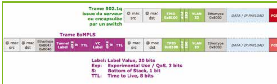
Figure 2 : Trame EoMPLS over Ethernet.
